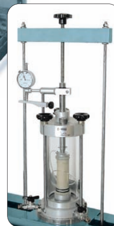
28-WF0493 Detail of the upper frame with the top knob to adjust and level the position of the beam device conforming to the different triaxial cells. The base plate is also suitable for other makes of triaxial cells provided that they are equipped with a centring hole 13 mm dia. by 3 mm deep
