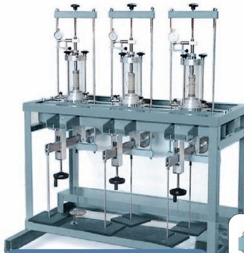
28-WF0493 complete with triaxial cells, dial gauges beam loading device and weights
