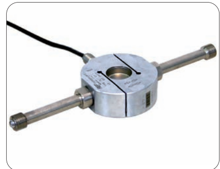
Detail of 27-WF0377/ST, 5 kN load cell
