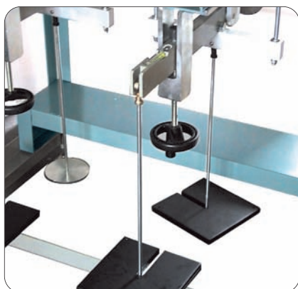
Detail of the 28-WF0493 10:1 beam loading device
