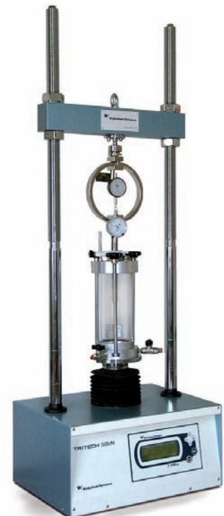
TRITECH 28-WF4005 fitted with standard triaxial cell 28-WF0410/A load ring and dial indicator
