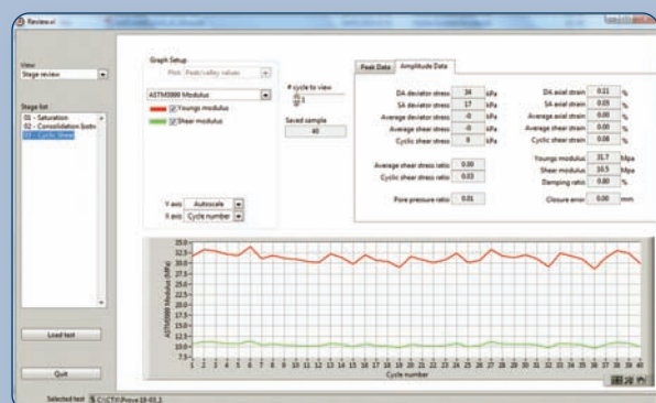
Cyclic shear Young's modulus and shear modulus are monitored during the cyclic stage against the number of cycles.
