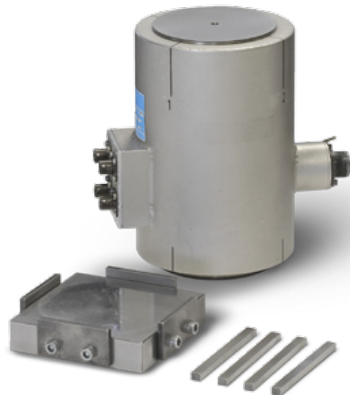
82-E0105/1. Strain gauged column. Carrying case included.
