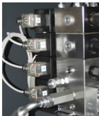
50-C20E82 fitted with 50-C10D/3F and 50-C20E/4F hydraulic valves for connection and control of a third and fourth frame
