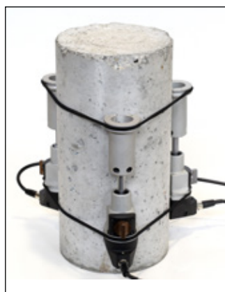
Concrete cylinder fitted with three Compressometer-extensometers 50-C0222/F
