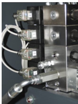
50-C10D/3F and 50-C20E/4F hydraulic valves for connection and control of four frames
