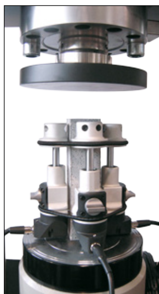
Cement prism fitted with three Compressometer-extensometers 50-C0222/F
