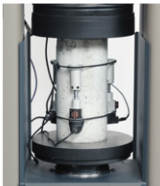
Three compressometer-extensometers (55-C0222/F) fitted to a cylindrical specimen during compression stage.
