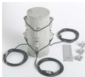
Three compressometer-extensometers (55-C0222/F) fitted to a cylindrical specimen (150mm diameter x 300mm high) ready for elastic modulus test.
