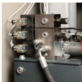
Detail of 50-C10D/3F valve to control up to three frames. Active frame selection via console display/software
